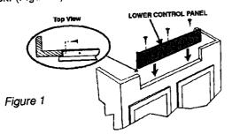
Position unit in the Countertop Cutout. Main Control Panel should overlap top of Lower Control Panel as shown. (Figure 2).
